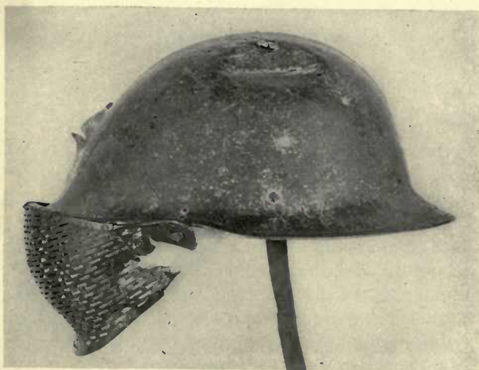
Fig. 48. Dunand helmet, showing result of tests
