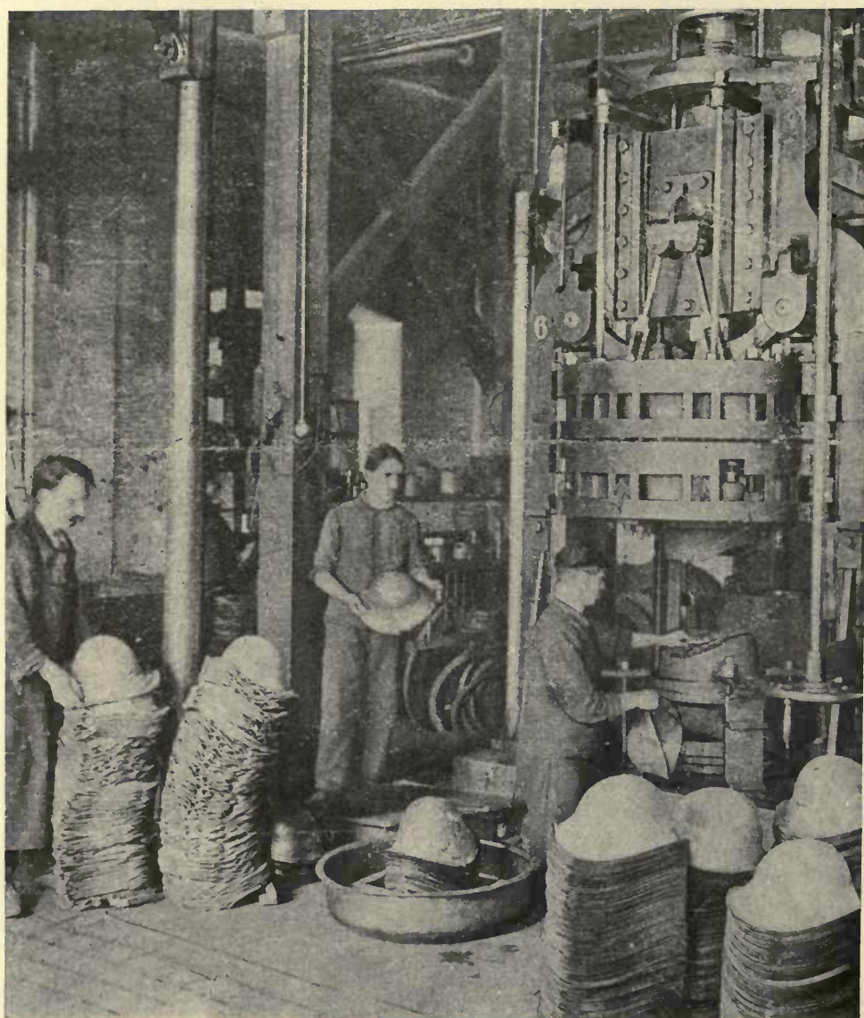
Fig. 126. Swiss standard helmet in process of manufacture
