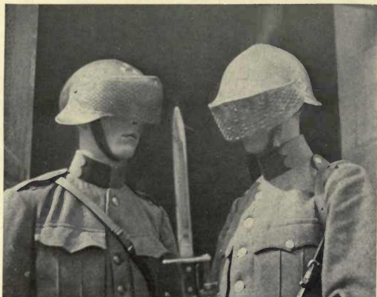
Fig. 123. Swiss experimental visor in place
