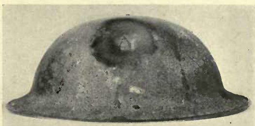
Fig. 86. British helmet showing indentation caused by glancing machine gun bullet
