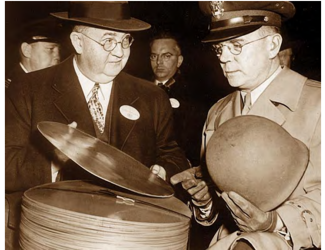
FIG 5. Carnegie-Illinois Steel Corporation - During a plant tour, a finished M1 helmet is shown in comparison to the helmet discs from which it was fabricated. (Credit: ACME -20 March, 1943- Author's Collection)
