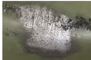
FIG 1. Typical example of the damage done to a M-1 helmet as a result of exposing the lot number in an attempt to maximize profit through perceived manufacture date.
