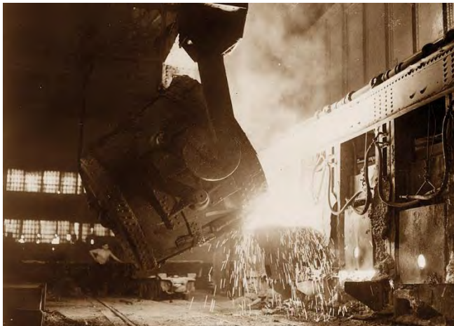
FIG 3. Carnegie-Illinois Steel Corporation - Giant ladle pours molten steel into an open-hearth furnace. (Credit: ACME-14 June, 1940 - Author's Collection)
