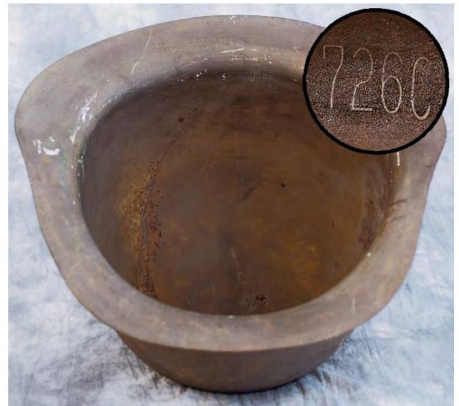
FIG 2. McCord M-1 helmet body after initial 7-inch draw prior to the trimming operation. Note Visor stamp 726C (Credit: Author's Collection)
