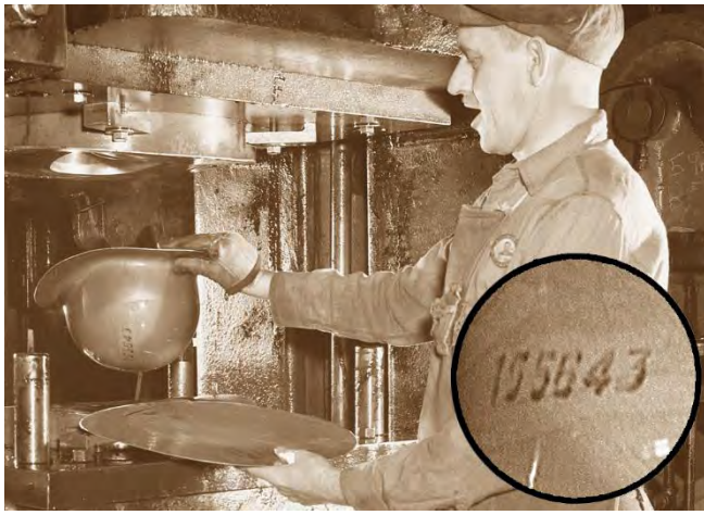
FIG 9. McCord Radiator & Manufacturing Co. - Manganese steel discs from Carnegie heat of steel No. 155643 are formed into a helmet in a single operation at one of many drawing presses. (Credit: Library of Congress-April, 1942)
