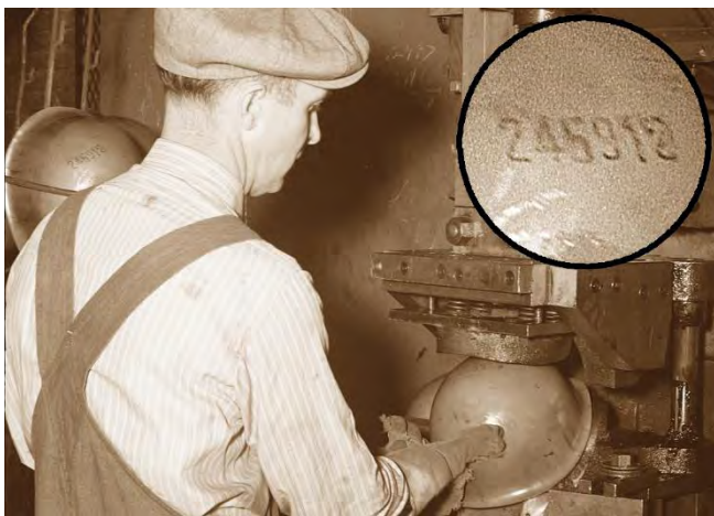
FIG 11. McCord Radiator & Manufacturing Co. - A helmet visor from Carnegie heat of steel No. 245912 is "cold-worked" in a "spanking" operation, which bends the visor down a small degree. (Credit: Library of Congress-April, 1942)
