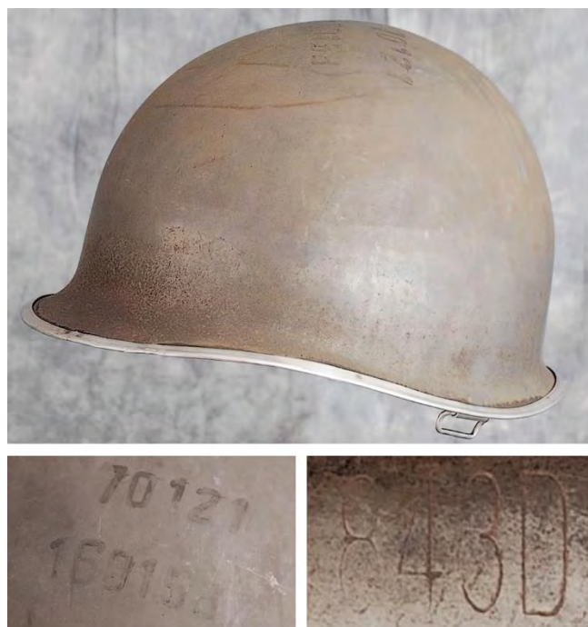
FIG 8. Carnegie-heat of steel No. 160158 received at McCord under lot No. 843. Carnegie-lift No. 70121 was assigned the letter "D" by McCord indicating it was the 4th lift of heat 160158 received. (Credit: Author's Collection)
